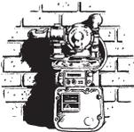
This winter please check, on a regular basis, your outside gas meter and regulator to make sure that no ice builds up on either. The gas regulator is a disc shaped device usually installed near the outside wall of your house in the piping connected to
